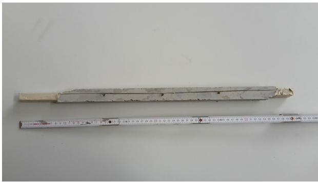
Fig. 6 Cement-coated test specimen from the CEM batch with epoxy resin protection at the clamping area
