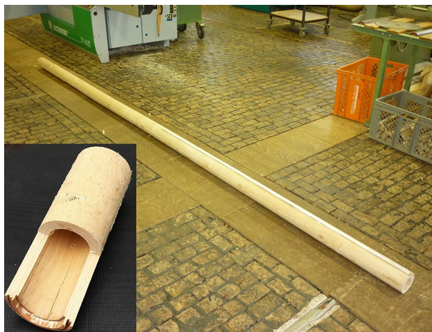
Fig. 1 4000 mm LVL hollow cross section with 100 mm outer diameter
