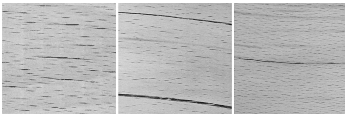
Fig. 3 Drying cracks running parallel to the spindles formed by the medullary rays
