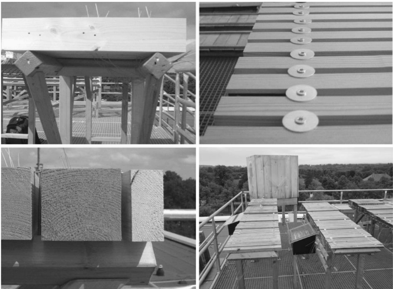
Fig. 1 Outdoor exposure of specimens. a Minimized contact area between specimen and bearing through rhombic supports. b Samples mounted with screws and washers. c Side shelter boards. d Set-up overview (Photo: Mehlich 2009)
