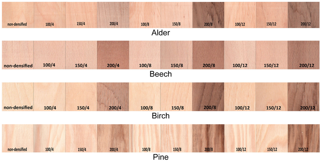
Fig. 1 Visual appearance of the surface of alder, beech, birch and pine veneers, non-densified and densified at different temperatures (°C)/ pressures (MPa)
