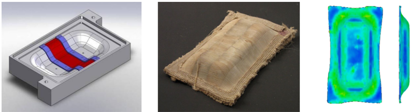
Fig. 11 Bottom part of the mould ( left ), end grain plate made of cottonwood with textile structures ( middle ) and illustration of FE-shaping with occurring shear stress ( right )
