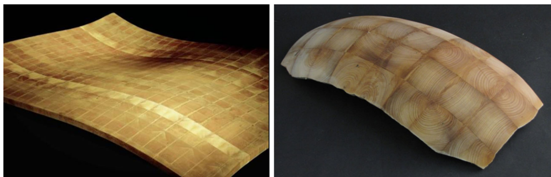
Fig. 12 Examples of moulded end grain boards of 900 \times 800 \times 20 \text{ mm}^3 “wave” and 500 \times 250 \times 10 \text{ mm}^3 “fender” made of lime
