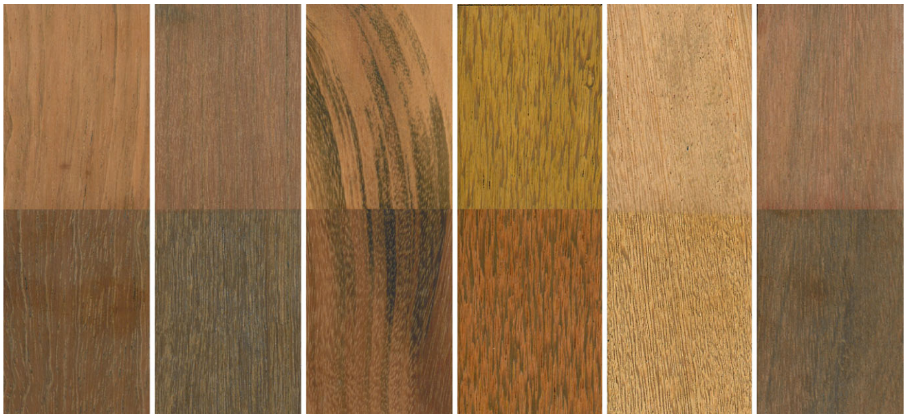
Fig. 1 Visual comparison of contrast among the exposed and non-exposed surface (from left : jatoba, massaranduba, tigerwood, amargoso, pedra, vermellho; upper half —unexposed, lower half —exposed for 144 hours)
