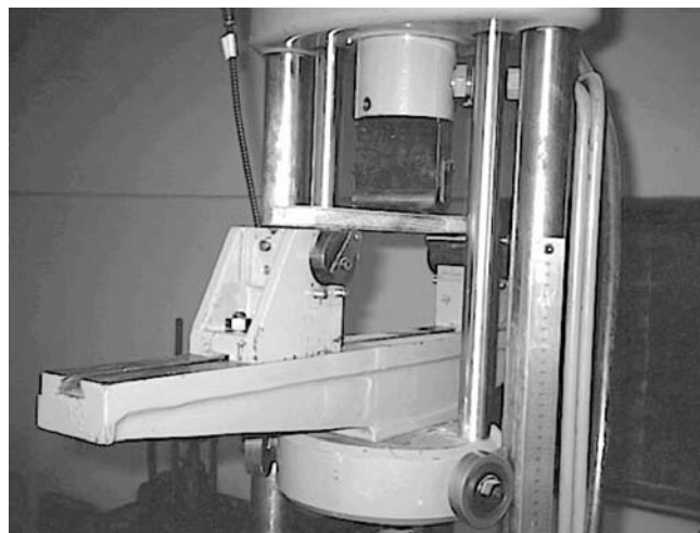
Fig. 2 MOR and MOE test set-up (Losenhausen test machine)
