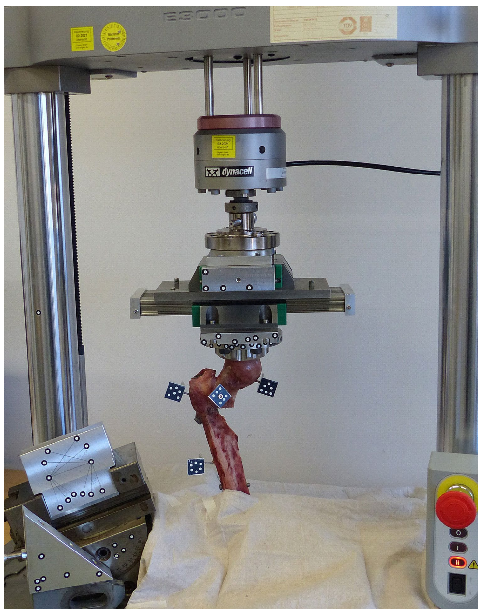
Fig. 2 Mechanical loading of the specimen via a conical load applicator attached to a multi-directional bearing plate and the machine actuator. Reference marker clusters defined the alignment of the coordinate system and interfragmentary motion was analyzed based on four marker flags attached to anatomical landmarks
