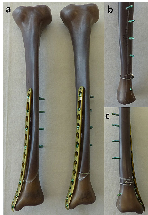
Fig. 1 Spiral fracture of the distal tibia treated with a metaphyseal locking plate and with a supplemental cable cerclage (a). The plate was instrumented with four 5.0-mm locking screws (bicortical) proximal to the fracture gap and one 5.0-mm (bicortical) and all four 3.5-mm locking screws (monocortical) distal to the fracture gap. View from lateral (b) and posterior (c) on the fracture zone with supplemental cerclage fixation
