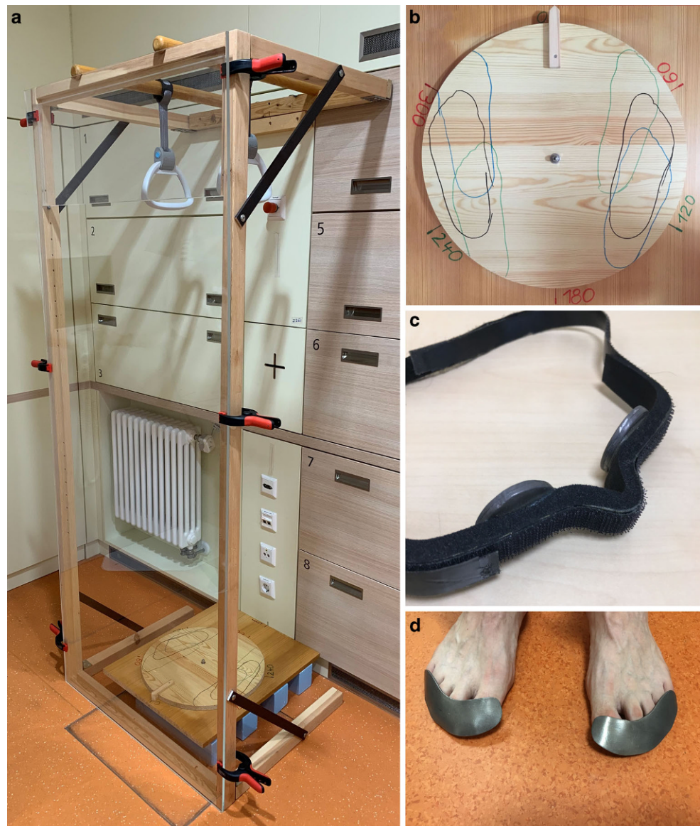
Fig. 1 Patient positioning. a Construction for patient positioning. b Rotatable plate with footprints for different treatment angles. c Shielding of eyes. d Shielding of nail beds
