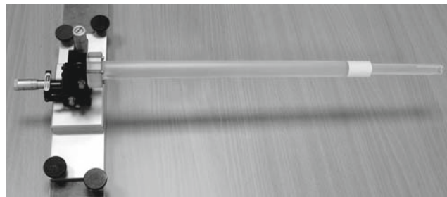
Figure 1. Photograph of the Elekta Ball Bearing Phantom. The metal sphere at the end of the Perspex rod may be positioned precisely with a three-dimensional translation stage. Markers on the surface of the rod allow an accurate alignment of the center of the metal ball onto the room lasers.
