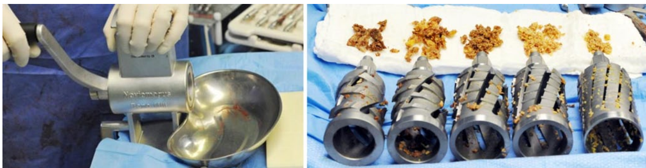
Fig. 1 ▲ Commercially available bone mill with five different drum sizes. The particles shown have cross sections from 1×1 to 8×8 mm and mean lengths from 1 to 15 mm [33]
