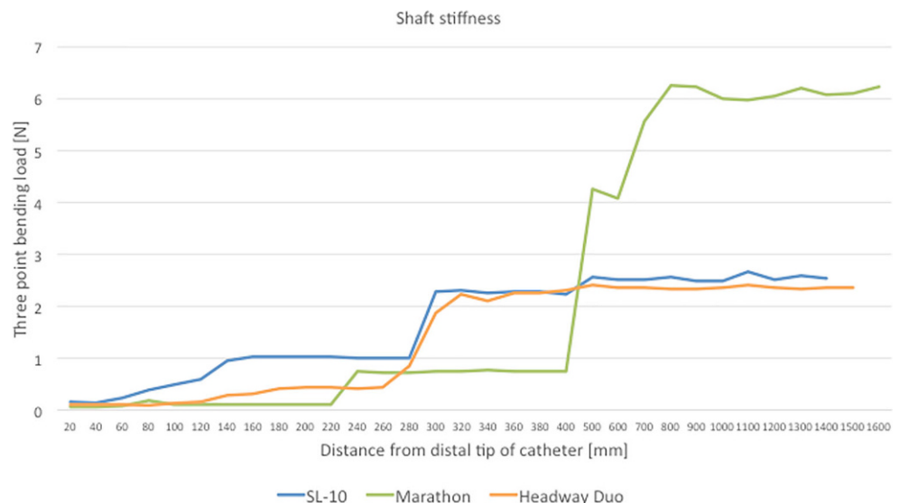
Fig. 6 Flexibility of the proximal shaft of each microcatheter
