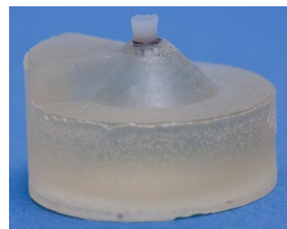
Fig. 4 ▲ Adhesive cylinder on embedded bracket. These were used to test shear bond strength at the bracket–adhesive interface.
