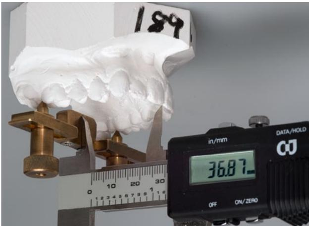
**Fig. 3** ▲ Device used to stabilize the caliper from sliding sideways.
