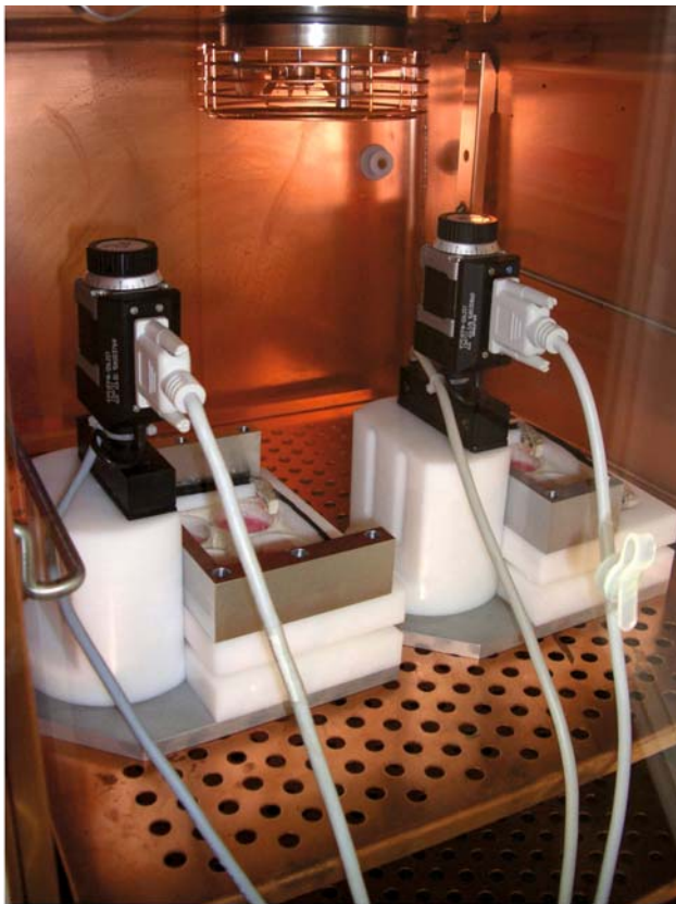
Figure 1. Strain devices used to apply cyclic tensile strain to PDL cells in an incubator.
