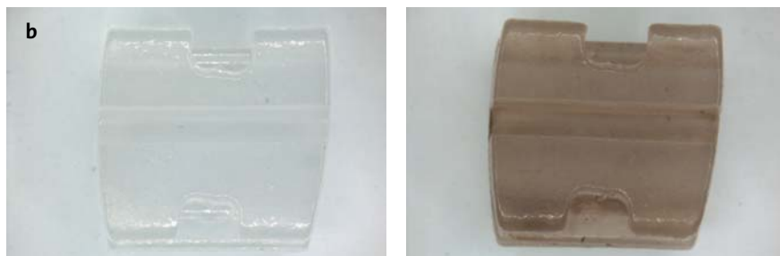
Figures 6a and 6b. Comparison of control brackets (on the left) to those immersed in black tea (on the right) on day 25: a) Aesthetic-Line® brackets, b) Ceramic 20/40 M brackets.
