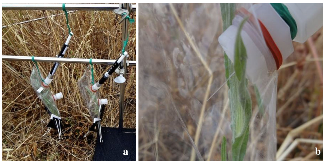
Fig. 2 Field setup: a in situ volatile collection of C. solstitialis using a Teflon ® Bag and SPME, b close-up photo of exposed SPME fiber
