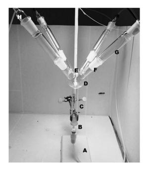
**Fig. 1** Major parts of the four-choice olfactometer: Retort stand (A), Entry area for insects (B), Central tube (C), Bulb (D), Hemispherical depression (E), Olfactometer arm (F), Extension tube (G), and Connector tube (H)
