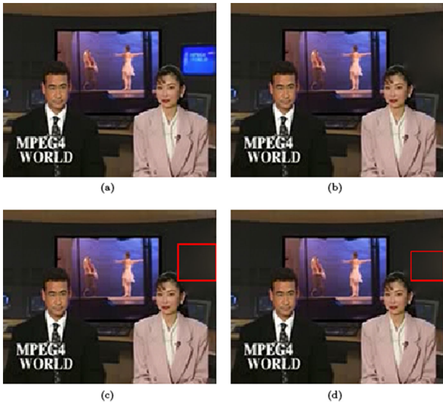
Fig. 14 Spatial tampering localization ability comparison between the proposed approach and the watermarking scheme [15]: (a) watermarked frame (b) tampered frame (c) localized tampering by the scheme [15] (d) localized tampering by our scheme
