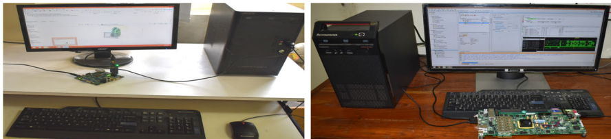
Fig. 14 Hardware Platform Test Setup; Left: on DSP Processor TMS320C6748, Right: on Zynq 706 All programmable SoC
