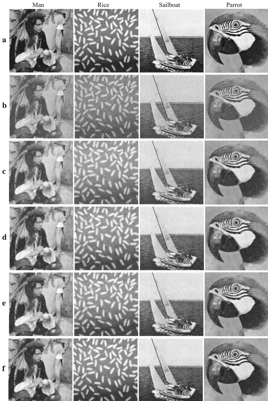
Fig. 4 Denoising performance with different models a original image, b noise image having N = 25 , c model in [60], d model in [30], e model in [38], f proposed model
