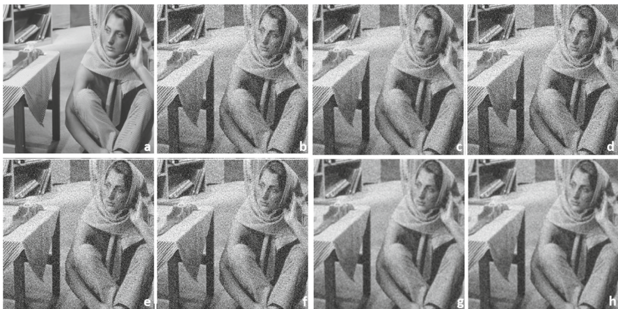
Fig. 7 Denoising results, here image is corrupted with GN, a barbara image, b image corrupted with GaussNs \sigma = 40 , c BFlt result, d gaussian filter result, e MedFlt 3 × 3 result, f MedFlt 5 × 5 result, g SG-BF filter result, h MSG-BF filter result
