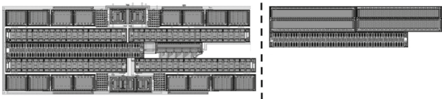
Fig. 16 Layout image of the symmetrical OTA using active mirrors ( left ) and classic mirrors ( right ). The first OTA on the left requires 3 times more area
