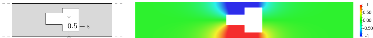
FIG. 5. Left: geometry of \Omega^\varepsilon . Right: real part of a trapped mode for \varepsilon = 0 and \sqrt{\lambda^0} \approx 1.9939
