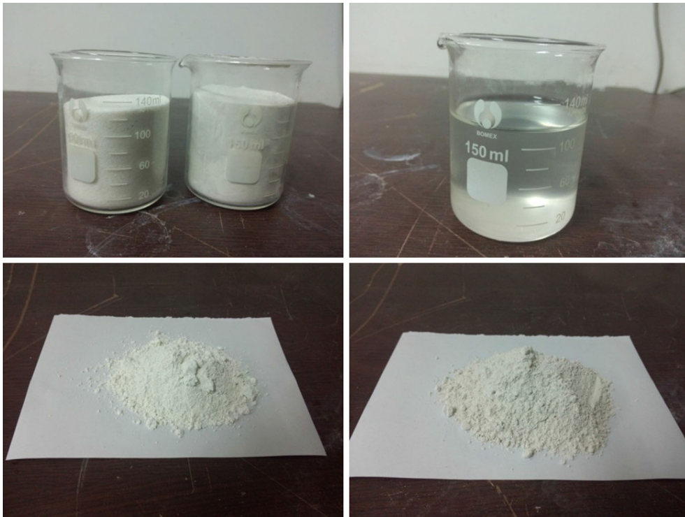
Figure 2 Materials used to construct synthetic samples (silica sands, sodium silica and clays)
