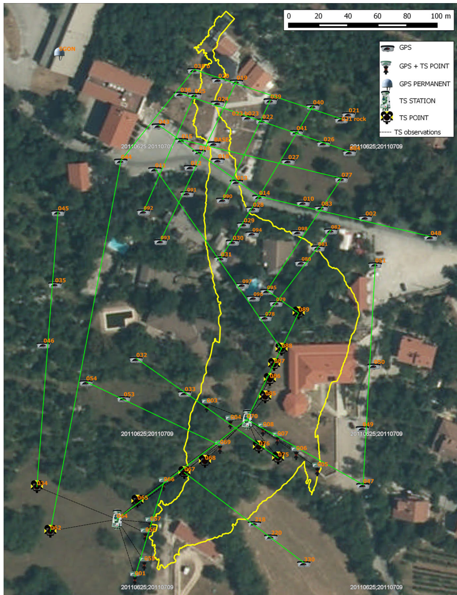
Figure 4 Scheme of observation of height with the different methods: RTK, Leica and Total Station
