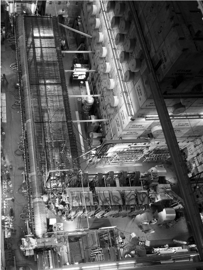
Fig. 4. A bird's-eye view of Nicholas Christofilos's Astron, around the time of its completion in 1963 at LLNL. The forty-foot electron accelerator sits horizontally at the bottom of the photo and the ninety-foot cylindrical tank on the left side is where the E layer was to be formed. Credit: Lawrence Berkeley National Laboratory, courtesy of Emilio Segrè Visual Archives, American Institute of Physics
