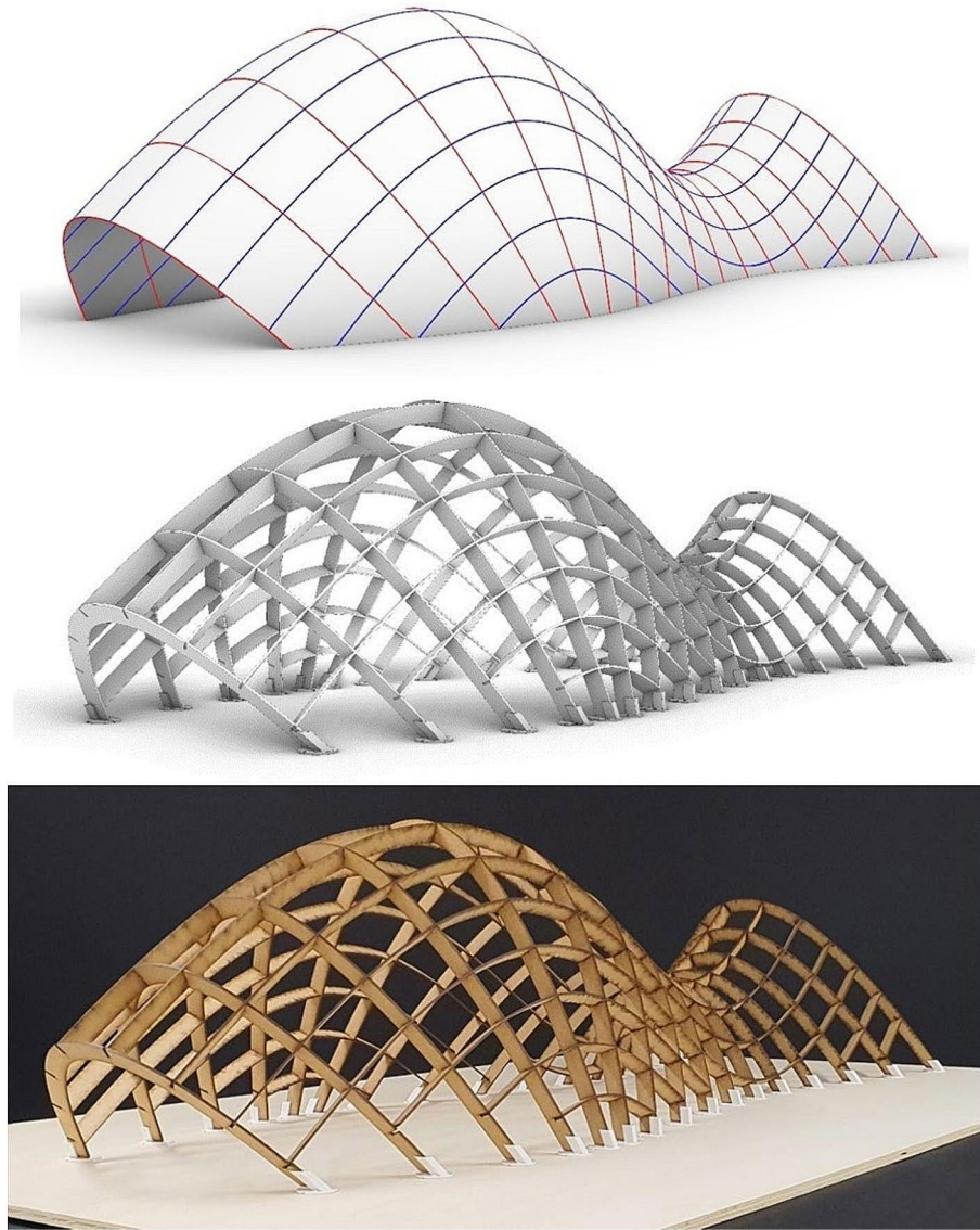
Fig. 12 Digital and physical models of a discretised Monge surface. Developable elements follow the PCL. Image: Pedro Nicolas Paduan Zahernski
