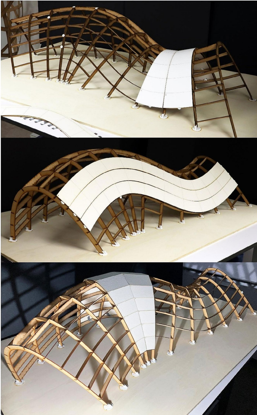
Fig. 13 Different approaches to an envelope system based on semidiscretised strips, parallel (above) meridian (middle) and discretized planar quads (below). Image: Pedro Nicolás Paduan Zahernski
