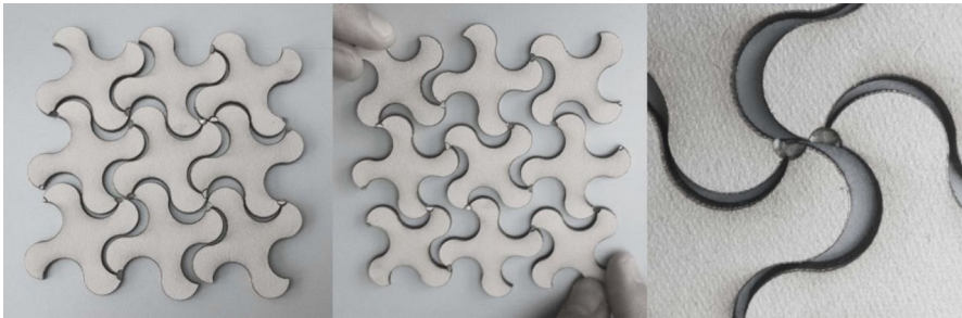
Fig. 15 One auxetic pattern built with meta-material. The different parts consist of three layers. On top and bottom of each part there is rigid cardboard which encloses flexible fabric in between. The fabric acts like a hinge (right)
