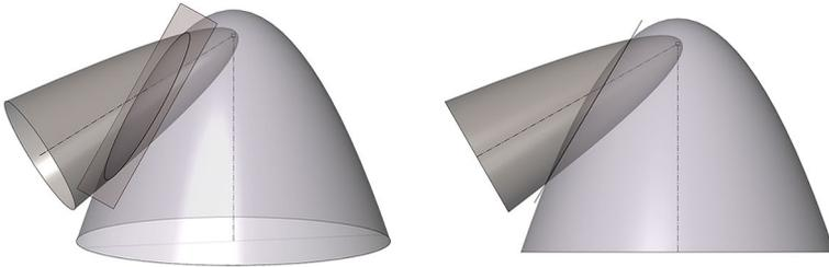
**Fig. 14** Paraboloid-Paraboloid intersection. The intersection between two paraboloids sharing the position of a focus at the same “real” point is a planar curve, and, in general, an ellipse. This supports the initial hypothesis. Source: Authors’ own
