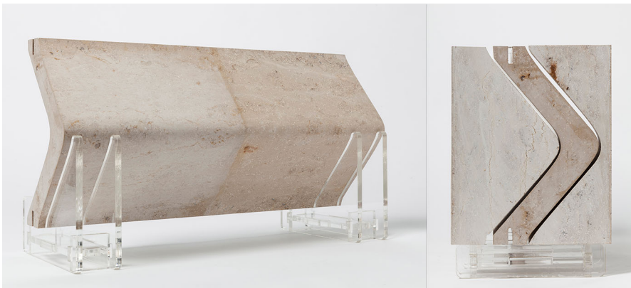
Fig. 24 The cut panel and the original stone block containing it
