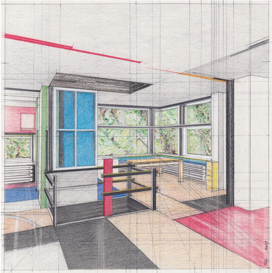
Fig. 5 Drawing in modular perspective of the interior of the house based on Rietveld's blueprints. The vantage point, here reproduced, is the same as in Rietveld's perspective drawing. The observer sightline runs almost on a golden line, whose points of interest are the following: a the corner of the balcony handrail behind the observer, and b near the corner post of the handrail in view (see Fig. 6). Image: the author and Brenda D. Macías
