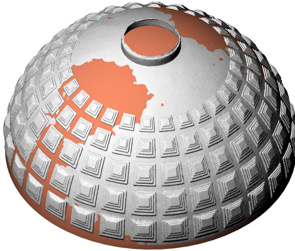
Fig. 4 View of the comparison between the survey model ( grey ) and the ideal model ( red ) (colour figure online)
