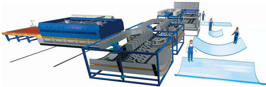
Fig. 43 Case study 3: diagram of CNC machinery used for glass panels production made by ruled portions (in the example, cylindrical surfaces), http://www.glaston.net/
