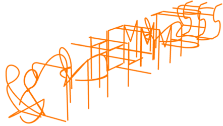
Fig. 26 Anamorphic curve produced by two plane curves in different construction plans. The set of both original curves is not readable when viewed as a three-dimensional object, but only as two projected views ( top and front )
