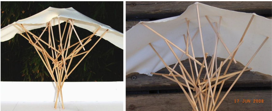
Fig. 11 Preliminary model to define a tree-like structure for the Melilla design
