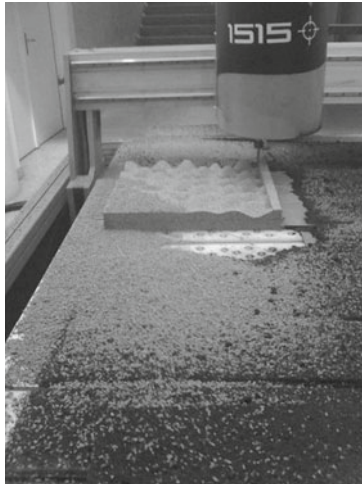
Fig. 2. Second day of the workshop, milling cork with a CNC router from Ouplan
