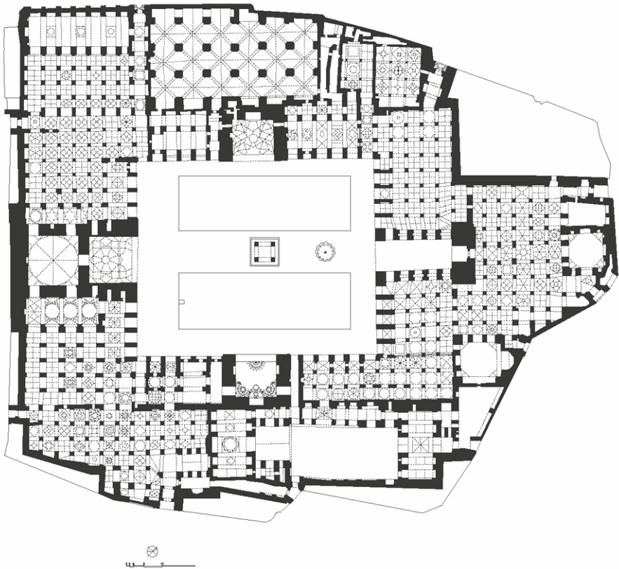
Fig. 2. Plan of the Friday mosque of Isafahan showing the reflective ceiling plan. Various asterisk-like geometric patterns of the shabistans make each individual vault space unique. Courtesy of Parsa Beheshti Shirazi
