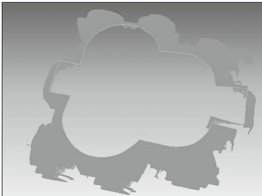
Fig. 18. Horizontal section obtained from the points cloud
