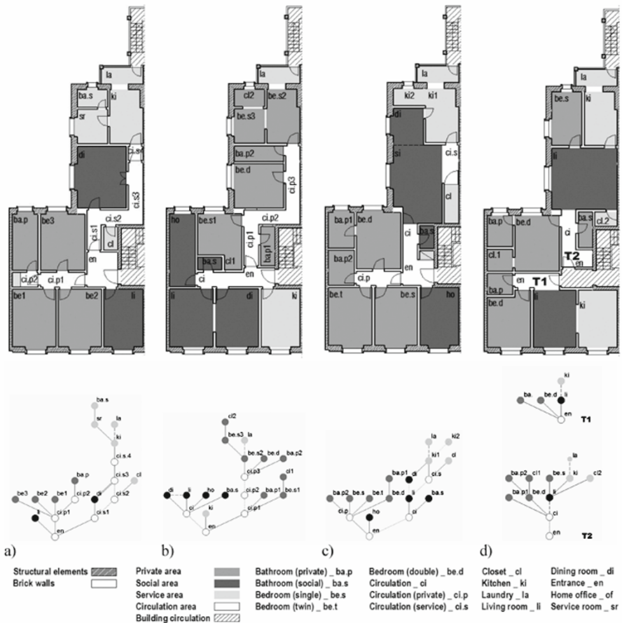
Fig. 5. Rehabilitation strategies: a) original dwelling; b) first strategy; c) second strategy; and d) third strategy. The top row shows the plans and the bottom row the corresponding justified graphs
