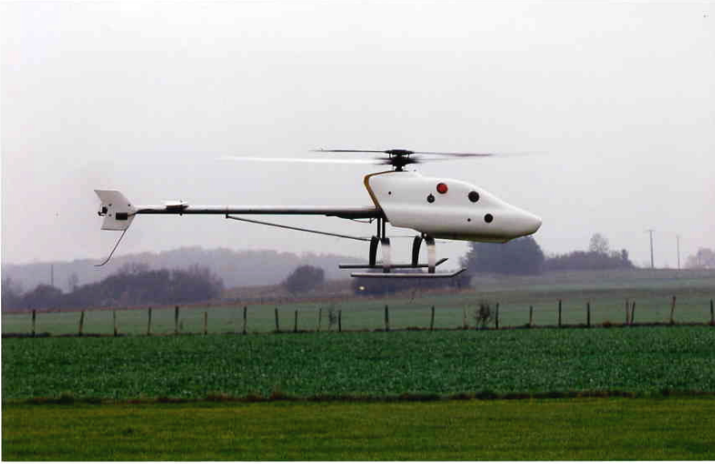
Fig. 3. Autonomous Helicopter with Microwave Radiometers for Emergency Mapping [1]
