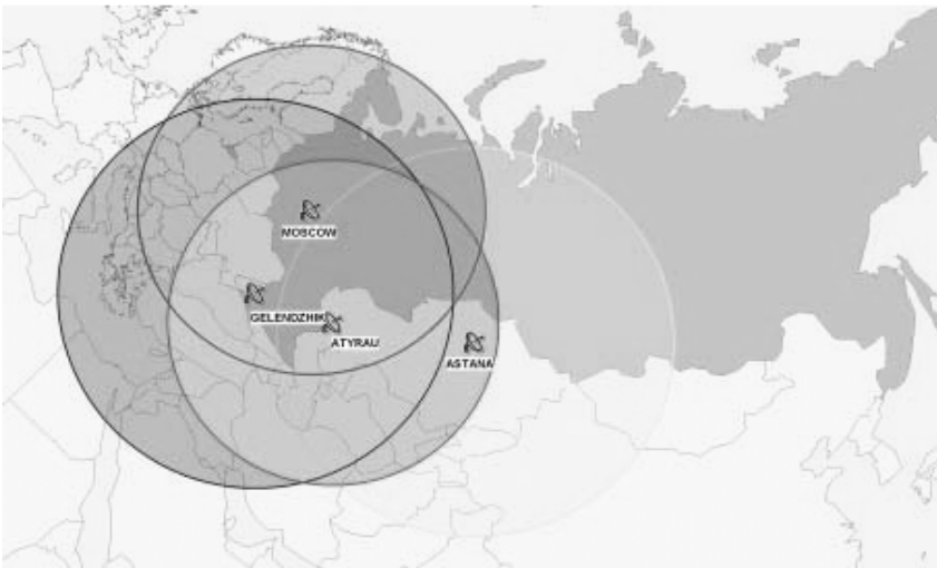
Figure 4. Network of RADARSAT-1 ground stations based on RADARSAT-1 terminal by R&D Center ScanEx
