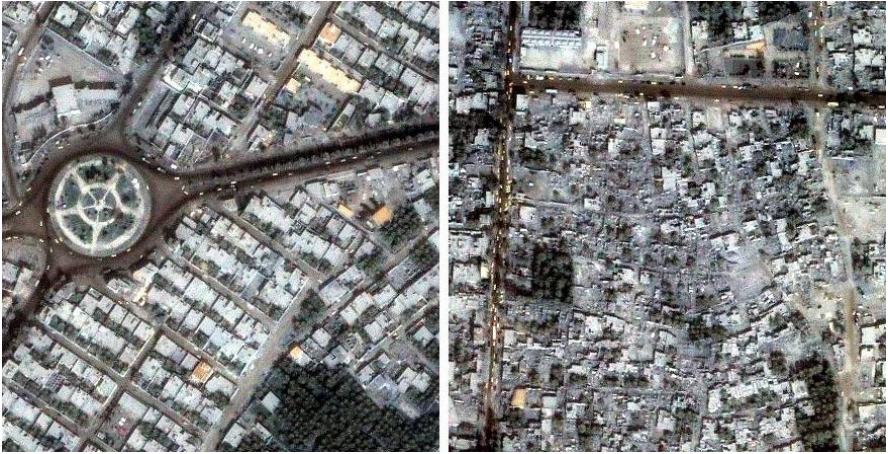
Fig. 8. Intact (left) and damaged (right) infrastructure after the Earthquake in Bam, South-Iran, mapped by IKONOS on December 27, 2003
