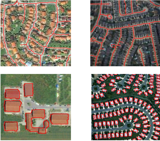
Fig. 6. Extracted road centerlines and building roof outlines (in red) overlaid on test images: (a) and (c) QuickBird, (b) and (d) IKONOS images
