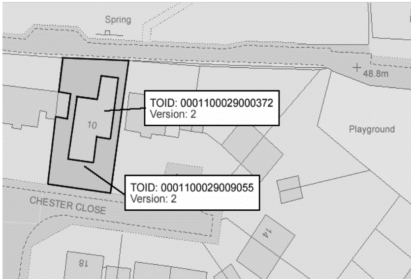
Fig. 2. Excerpt of OS MasterMap Topography Layer. Every geographic object has a unique TOID ® for data association
