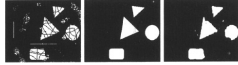
Fig. 2. Example for noise filtering. From left to right: sample noisy image, gold sample provided by the user, and filtered image by generated MM procedure. The result has a 96.77% similarity to the gold sample.
