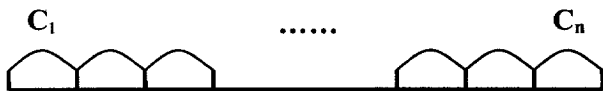
Fig.1. As for a digit sample, here are n 16-dimension-vectors. Every vector has 16 dimensions which are 16 MFCC after step 1.
