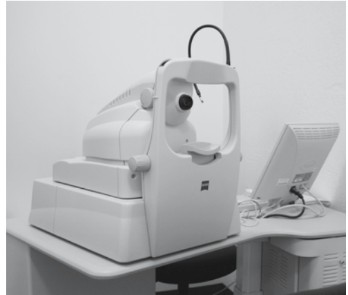
Fig. 1.3. Photograph of the latest generation Stratus OCT (Carl Zeiss Meditec Inc., Dublin, CA, USA). Both the table and the chin rest are adjustable to the patient's height. The movable fixation light can be placed in front of the contralateral eye to help the examination of eyes with loss of central fixation
