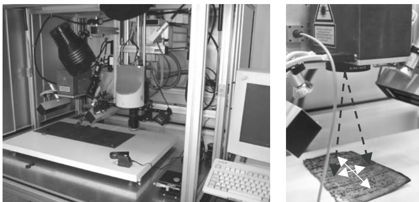
Fig. 4. Cleaning laser system (BAM Prototype). Remote control scanning principle
