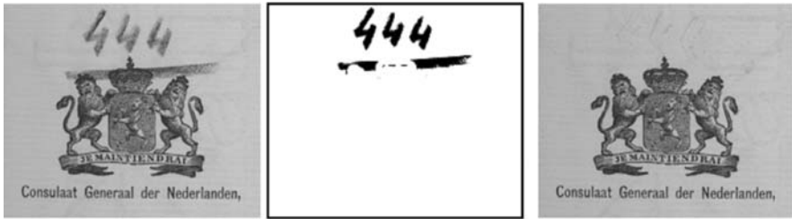
Fig. 3. Selective removal of chalk from paper ( left ) before cleaning the object, ( middle ) digital isolated black and white image and ( right ) the object after laser treatment
