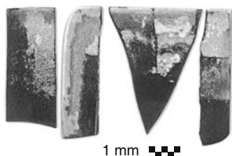
Fig. 1. Model glass with corrosion crust, partially cleaned with brushes (overview, transmitted light)
