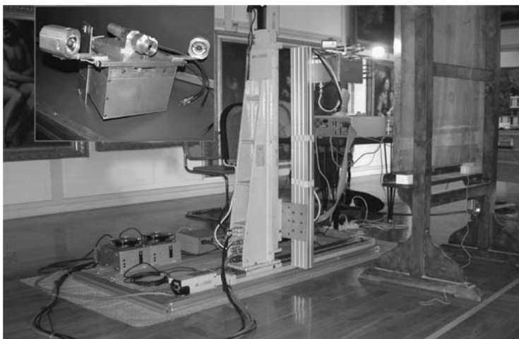
Fig. 1. The IR-Colour scanner in the Borghese Gallery (Rome) and the Optical Head
