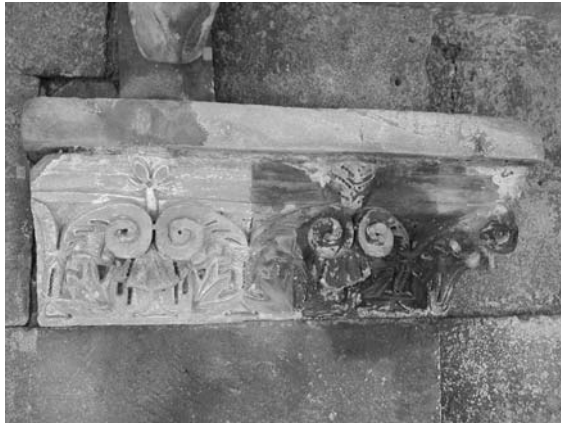
Fig. 2. Detail of a marble capital, partially cleaned by a Nd:YAG laser
