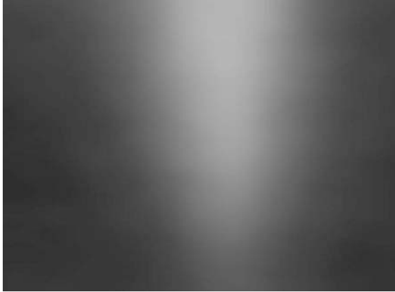
Fig. 4. Radiographic shadow of a steel pin in limestone generated by a miniature X-ray source located in a nearby hole
