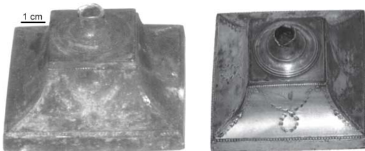
Fig. 1. The base of the candlestick before and after laser cleaning (one side with one laser source)
