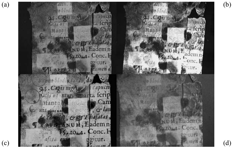
Fig. 2. Chaetomium on handmade rag paper ( \sim 1600 A.C.). Multispectral Imaging. (a) VIS reflectivity (b) fluorescence (c) IR reflectivity (d) UV reflectivity. Fluence 0.5\text{--}1.3\text{Jcm}^{-2} . \text{KMnO}_4 -bleached sample in lower right corner of each image
