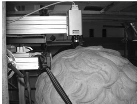
Fig. 3. The probe-statue fixing system
