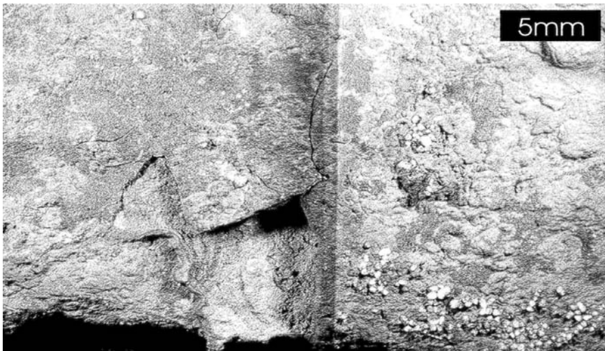
Fig. 6. Liquid film (ethanol) on the surface also removes silica grains; left : laser cleaned ( \lambda = 1064 \text{ nm} ) with ethanol liquid film; right : laser cleaned ( \lambda = 1064 \text{ nm} ) without ethanol liquid film
