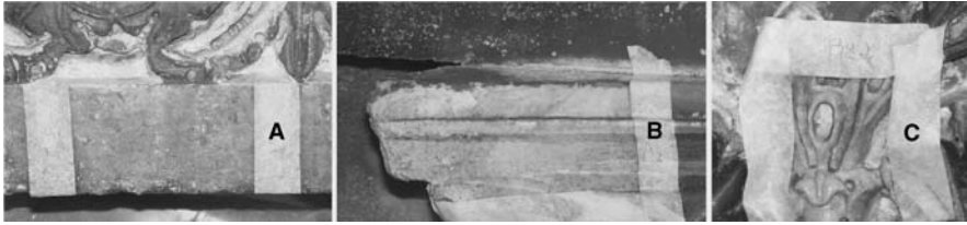
Fig. 5. Laser cleaning tests performed on flat and decorated surface of a façade with a Nd:YAG laser
