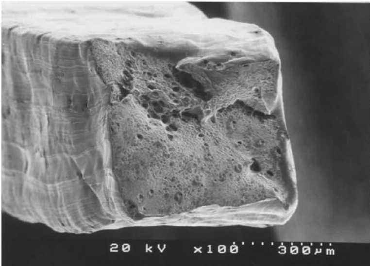
Fig. 8.6. Expanding ring dynamic fracture characteristics
