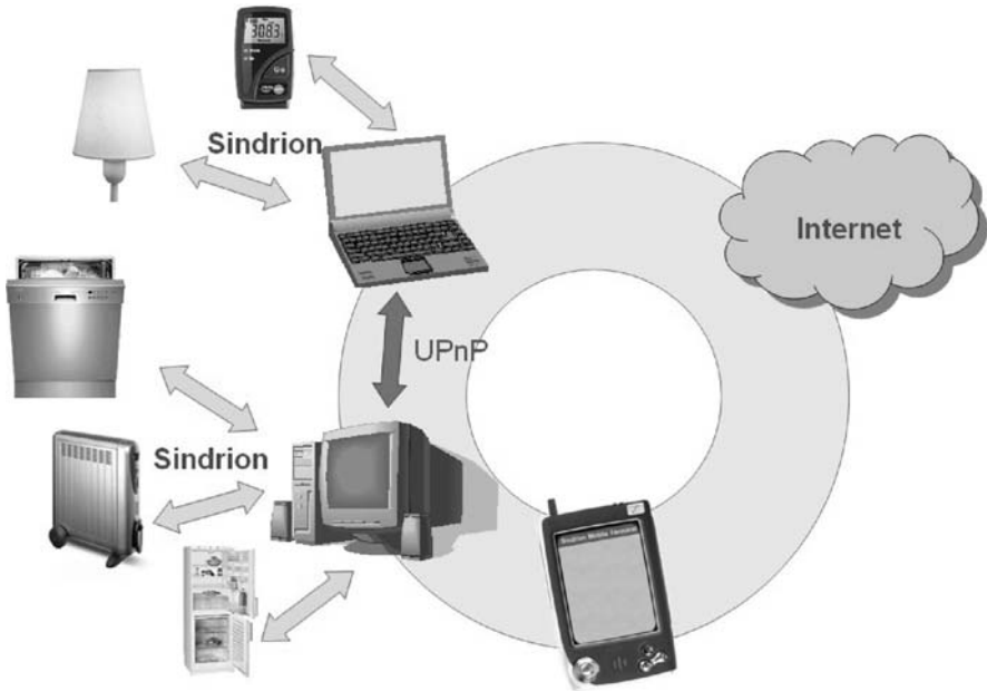
Fig. 7. Sindrion Transceivers as a part of a UPnP Distributed System
