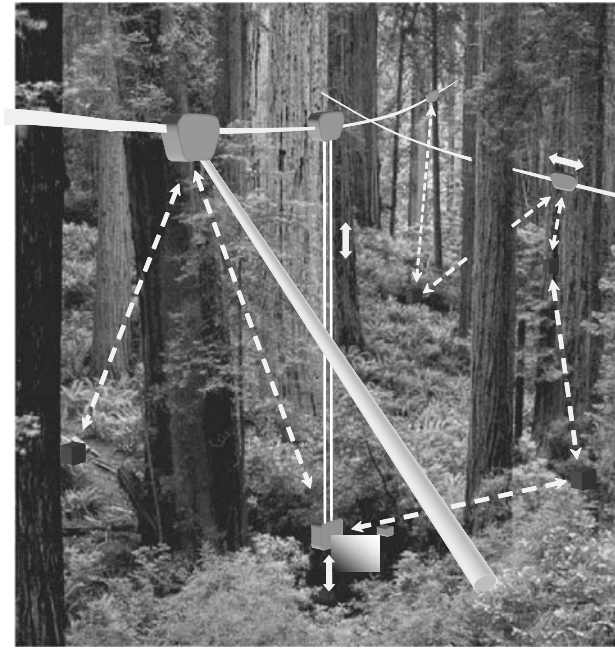
Fig. 1. Networked Infomechanical Systems (NIMS) introduces a hierarchy of fixed and mobile sensing nodes and infrastructure enabling access to complex, three dimensional environments. NIMS mobility provides novel methods for establishing self-awareness of sensing uncertainty. Further, examples of new NIMS distributed services include node transport, physical sample acquisition, energy harvesting and delivery, wireless network relay functions, and many others
