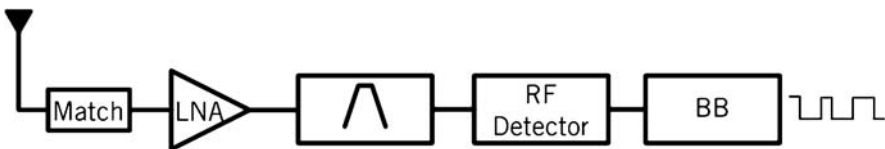
Fig. 7. TRF receiver architecture with envelope detector
