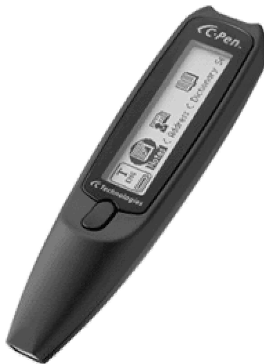
Fig. 2. The C-Pen from C Technologies AB (Courtesy of CPEN 2003)
