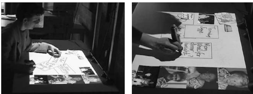
Fig. 2. Interacting with the FRIDGE prototype in a laboratory: manipulating electronic notes with a tangible user interface and using an electronic stylus strictly as a pen
