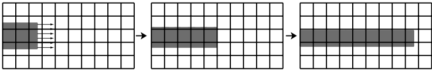
Figure 4.16. Deformation process obtained by the PE-FCM applied to the uniform tension problem.
