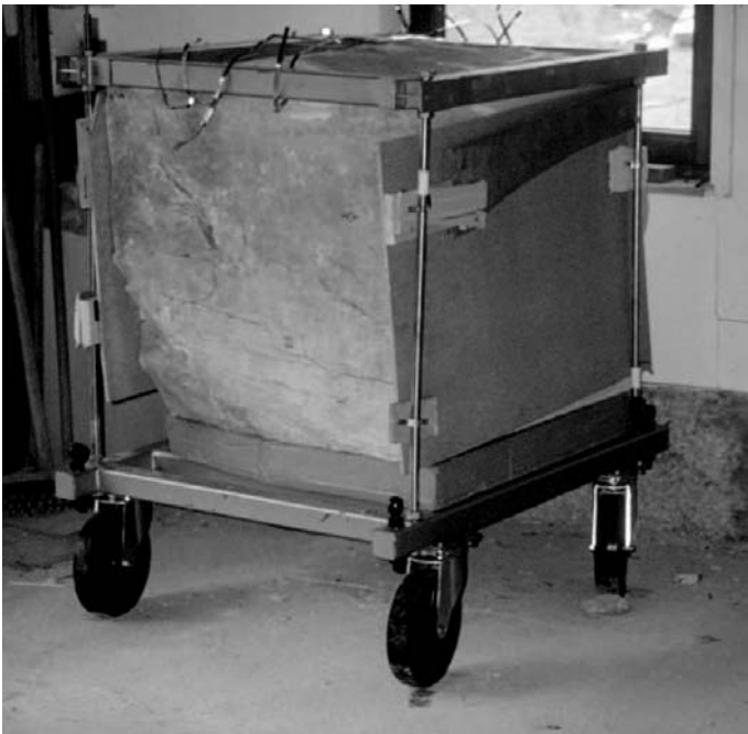
Fig. 4.14. 90 \times 90 \times 80 \text{ cm}^3 -block: Block sample on mobile platform.
