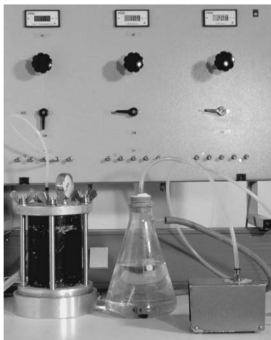
Fig. 3.8. Resin injection equipment (Baraka-Lokmane et al. , 2003).
