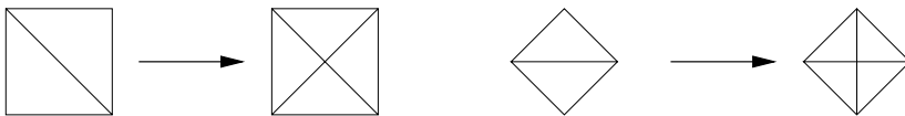
Fig. 4. Split sets corresponding to the two types of diamonds generated by recursive triangle bisection.
