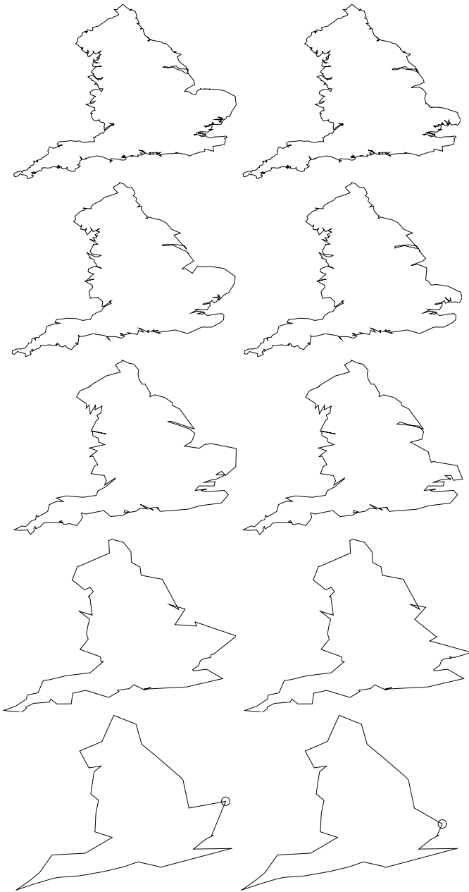
Fig. 5. Example: Local editing. The left side, top to bottom, is the reverse subdivided outline of England (585 vertices to 37 vertices). The right side, bottom to top, is the modified outline, reconstructed using the same errors as the left side. The circle indicates the modified vertex.
