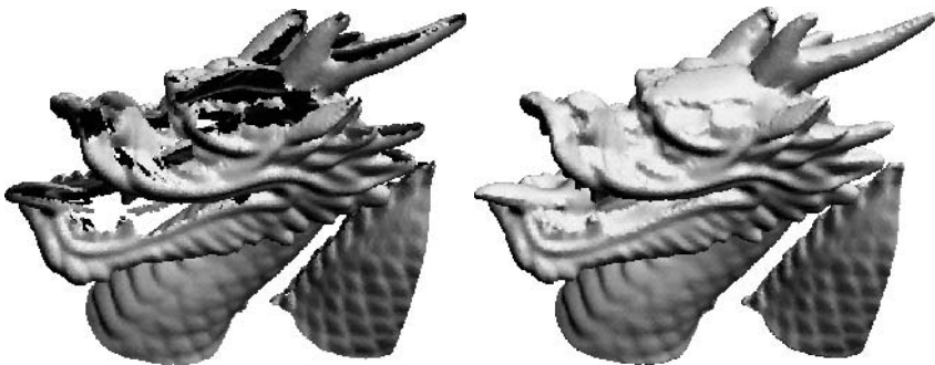
Fig. 2. Reconstruction of incomplete data obtained from range scans of the Stanford dragon model.
